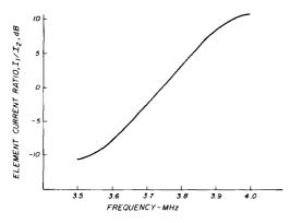
fig. 9. Calculated current ratio between the two dipoles of the parallel antenna.
